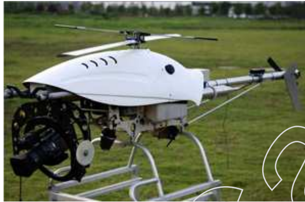
Two axes, stabilized camera mount. Stabilization is integrated with XP3.1 autopilot.
